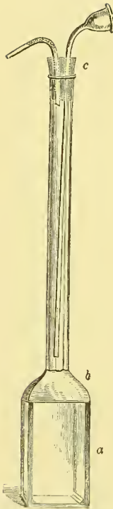
Apparatus made for examining the circulation in the branches of a proteus. The smaller tubes were for the purpose of supplying the animal with fresh water. p. 75.
